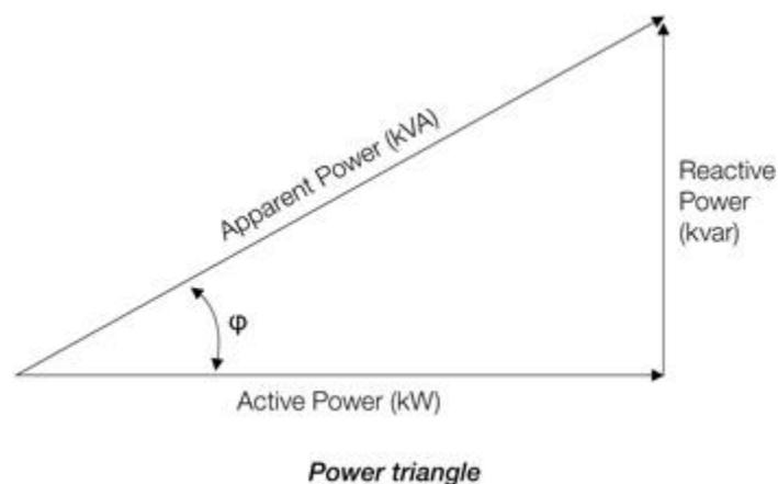
The relationship between kVA, kW and kVAR is non-linear and is expressed: as:  $kVA^2 = kW^2 + kVAR^2$
